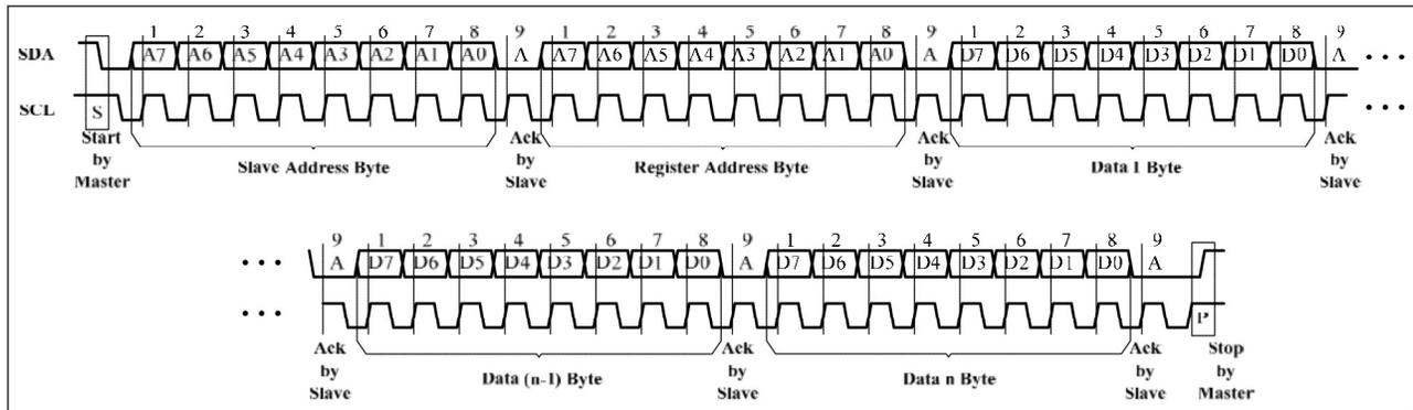
Figure 7 Writing to IS31FL3733B (Automatic Address Increment)
