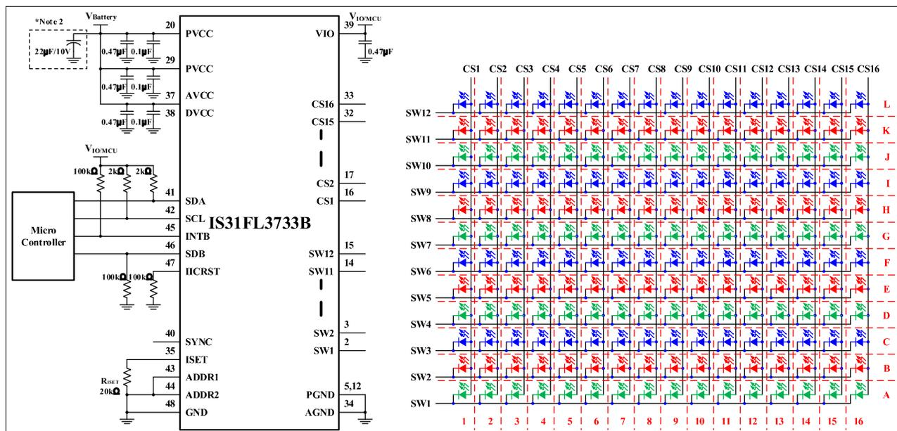
Figure 2 Typical Application Circuit (RGB)
