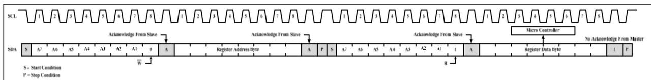
Figure 8 Reading from IS31FL3733B
