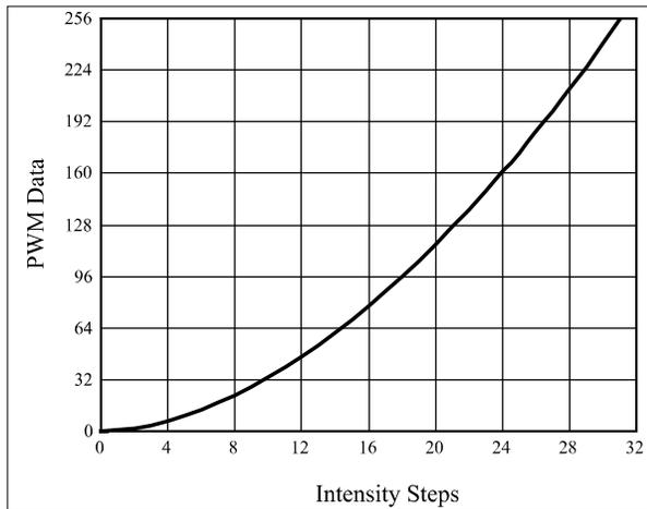
**Figure 13** Gamma Correction (32 Steps)
